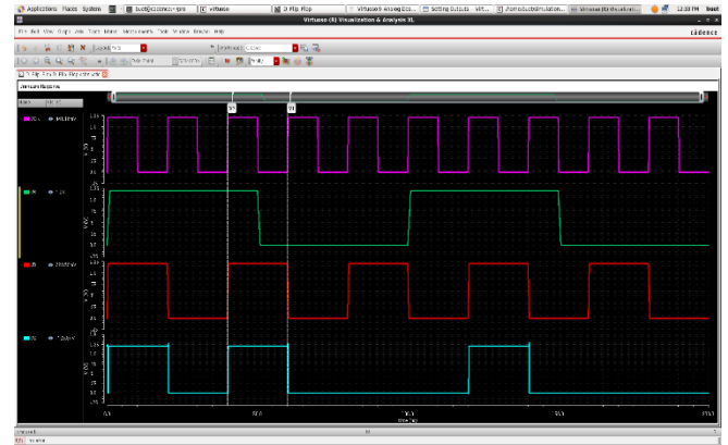
Fig. 6. Transient response when reset value is low.
